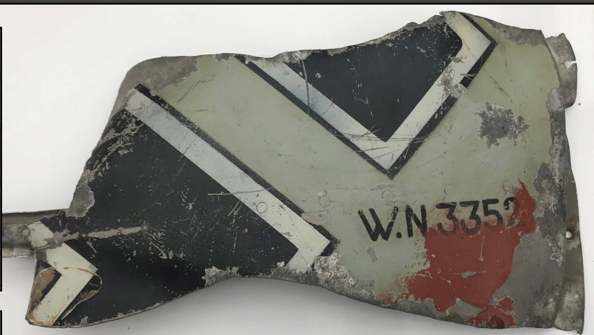
Part of the tail surfaces of the machine of Koepsell and Schmidt. On the inside, a protective coating in the shade RLM 02 is visible. On the outside, a red color is painted for unknown reason over the pale blue RLM 65. Photo: Stephen Newman
